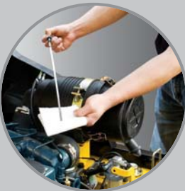
Quick and easy engine oil check
