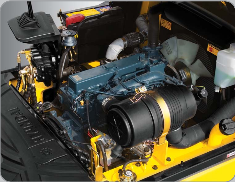
Centralized design for easy service! An ideal arrangement of component parts ensures easy access and convenience for maintenance.
